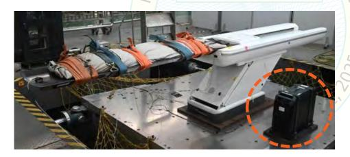
UUT was rigid base mounted with (4) M10 bolts, grade 8.8.
