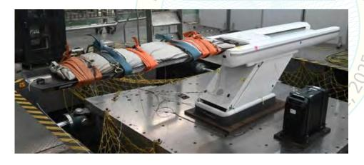
UUT was rigid base mounted with (4) M16 bolts, grade 8.8.
