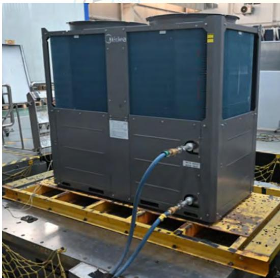
UUT was base mounted - isolated on LSLGRW600/III.JZD neoprene pads manufactured by Changzhou Songying Machinery Factory using (4) Grade 8.8 M16 bolts. Unit maintained structural integrity and remained operational per manufacturer requirement following shake table test. All contents were included in the unit per operating conditions.
