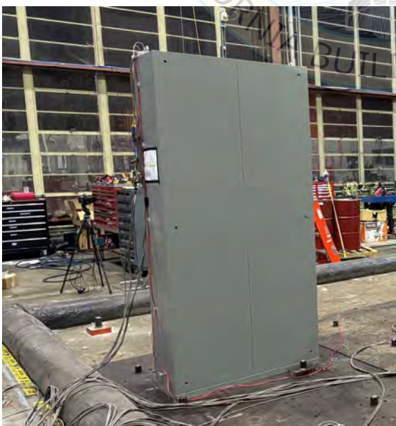
UUT10 mounted on the shake table
