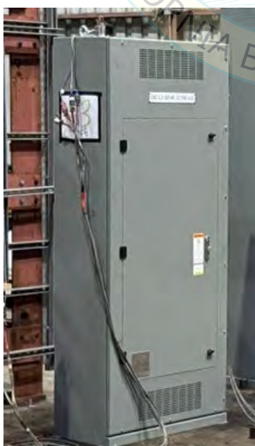
UUT9 mounted on the shake table
