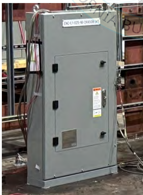
UUT7 mounted on the shake table
