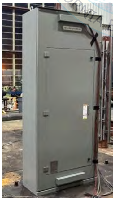
UUT5 mounted on the shake table
