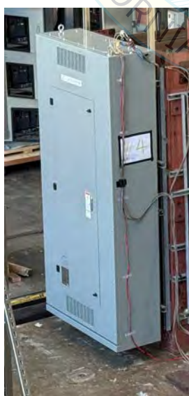
UUT4 mounted on the shake table
