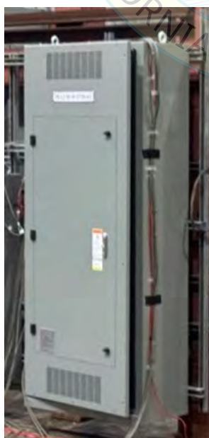
UUT3 mounted on the shake table
