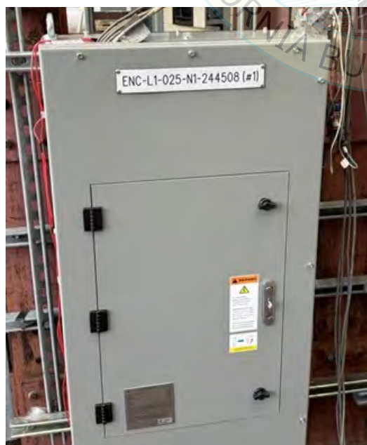
UUT1 mounted on the shake table
