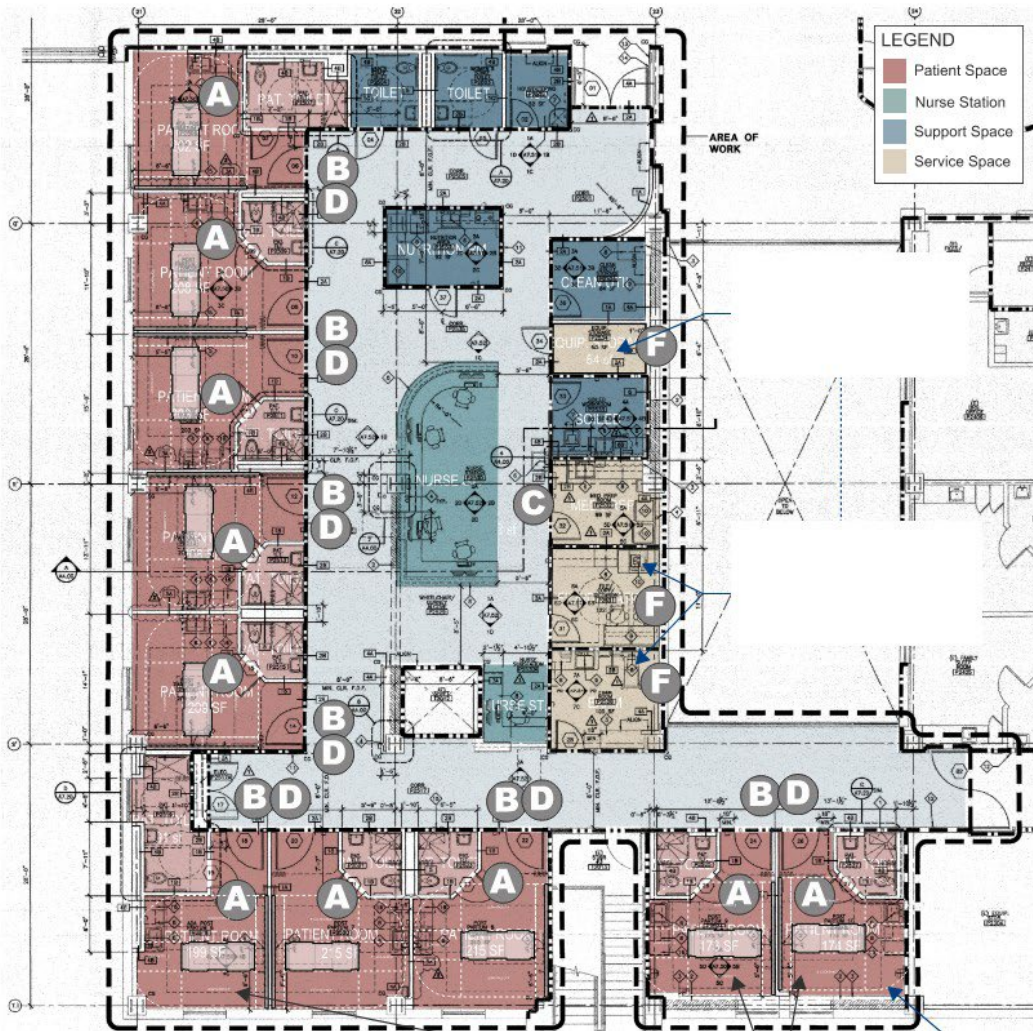
Figure 2: Example of a compliance diagram (Intensive Care Unit)
