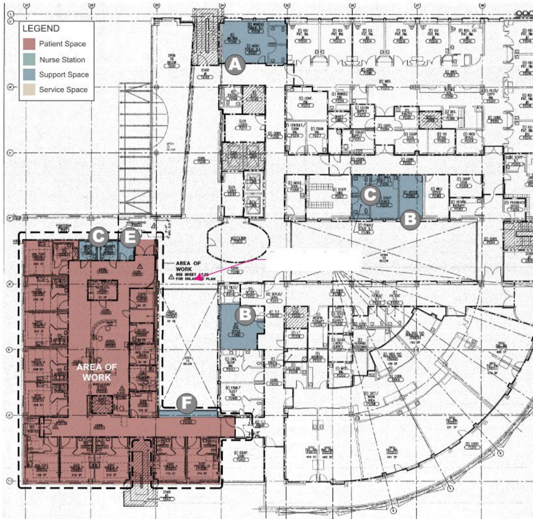
Figure 1: Example of a floor plan with area of work identified (Intensive Care Unit)
