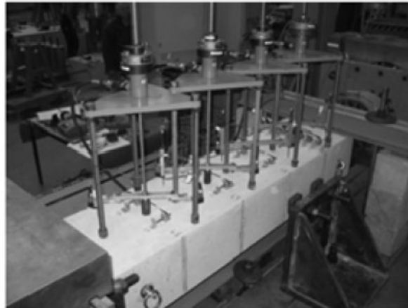
Fig. 7—Anchor loading setup for seismic crack cycling tests.
