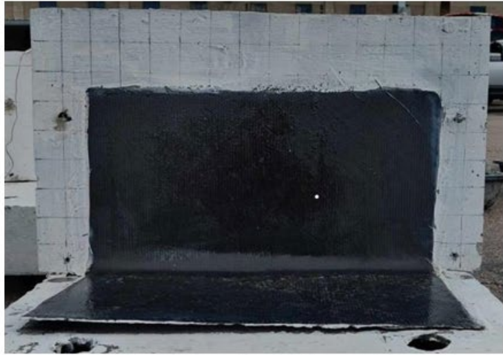
a. Debonding failure in SP8
