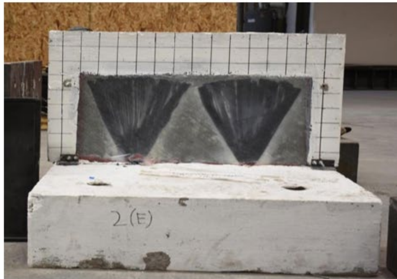
d. Failure at connection - SP12
