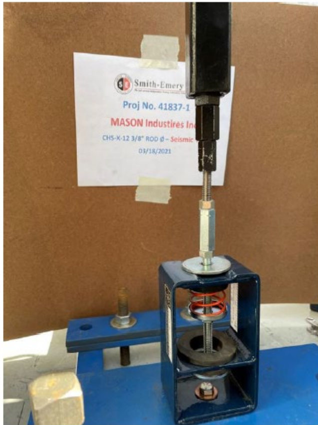
Typical Test Setup for CHS-X-12 3/8" Rod Ø: Vertical Configuration
