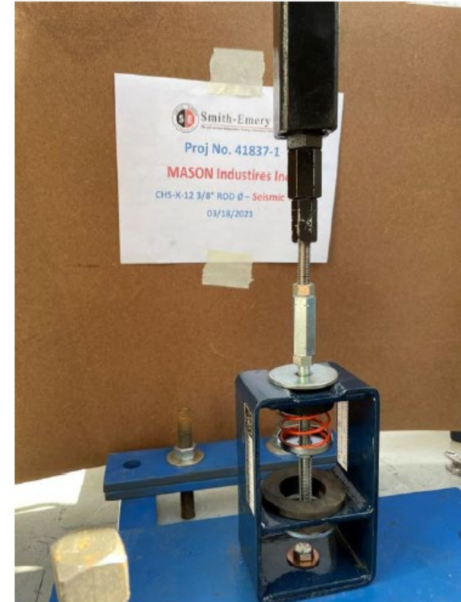
Typical Test Setup for CHS-X-12 3/8" Rod Ø: Vertical Configuration
