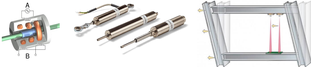
(b) examples of sensors which can be used to directly measure displacements
