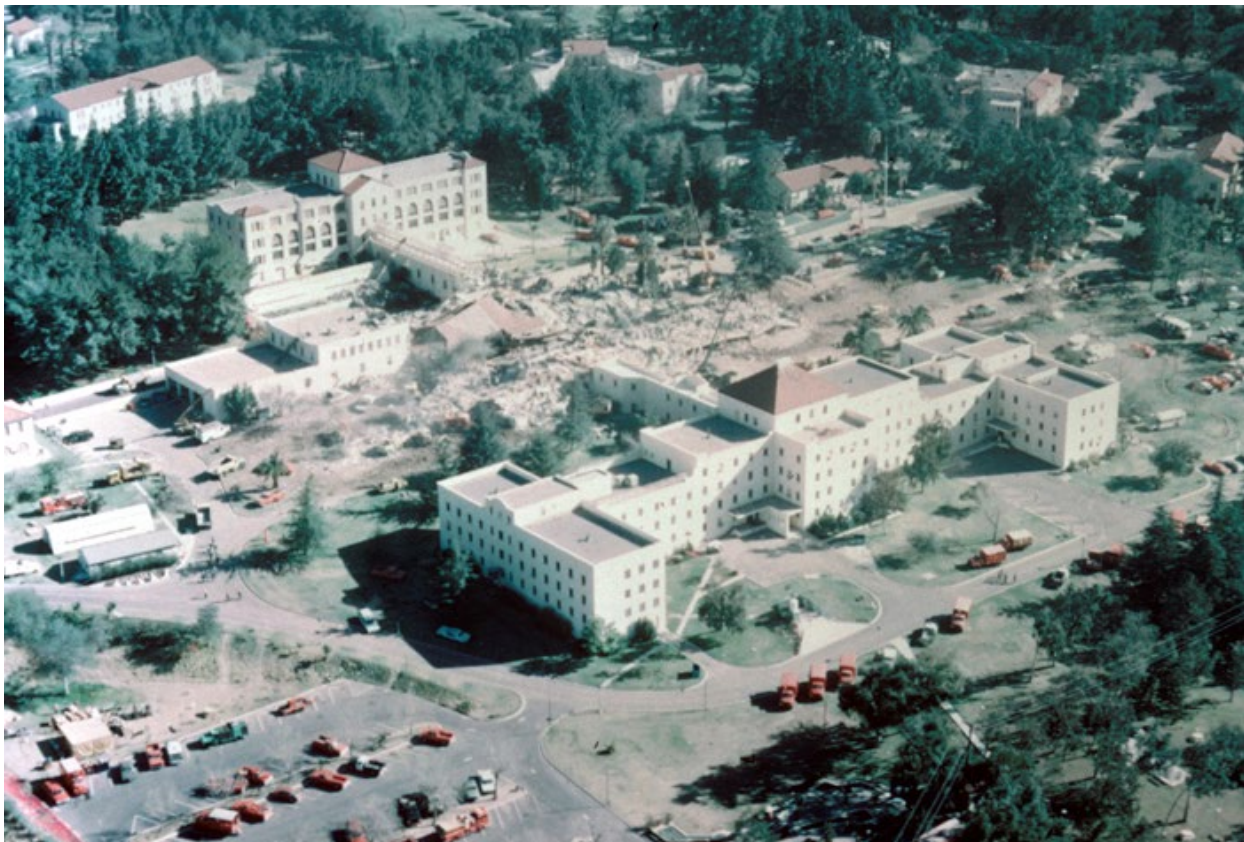
Figure 1. The 1971 San Fernando earthquake in southern California resulted in the collapse of Building-1 and -2 at the San Fernando VA Hospital and loss of 49 lives. (Source: USGS earthquake photo archive, available online at https://library.usgs.gov/photo/#/?category1=earthquakes&collection2=san%20fernando%20earthquake,%20february%201971 )
