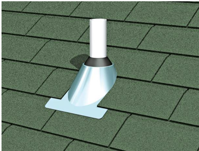
Shingles at Pipe Vent
