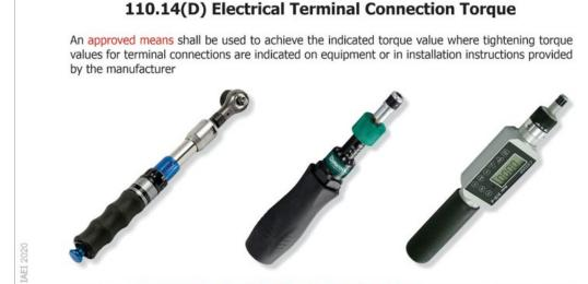
Examples of approved means of achieving the indicated torque values include torque tools or devices such as shear bolts or breakaway-style devices with visual indicators that demonstrate that the proper torque has been applied
