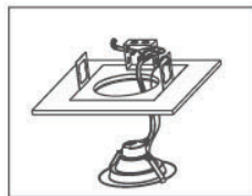
Bypass ballast & wire to j-box
