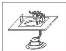
Bypass ballast & wire to j-box
