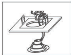
Bypass ballast & wire to j-box
