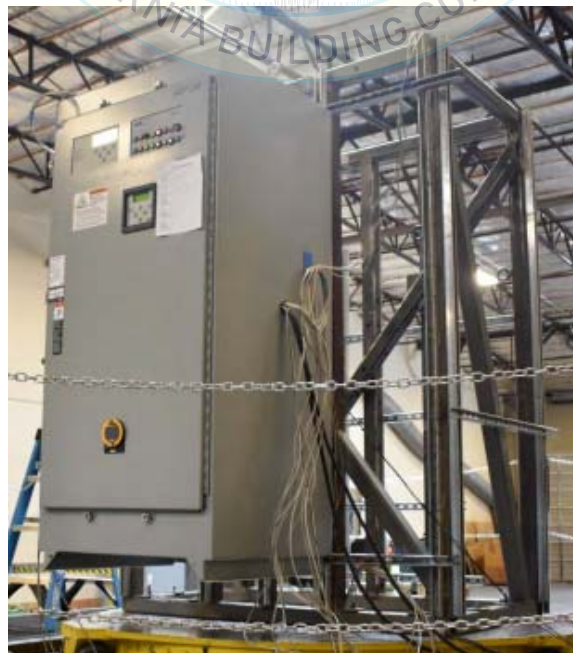
All units were filled with contents and maintained structural integrity and functionality after AC-156 test.
