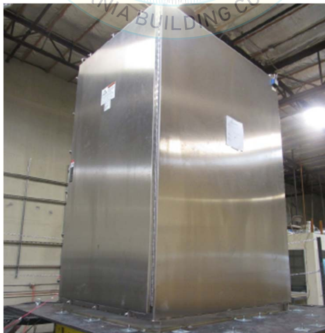
All units were filled with contents and maintained structural integrity and functionality after AC-156 test.
