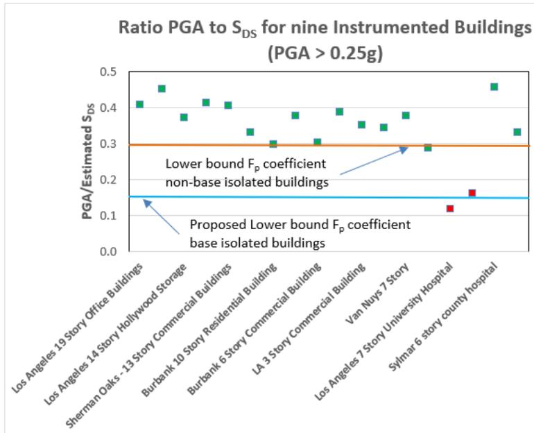
**Figure 10:** Comparison of PGA to the  $S_{DS}$  from nine instrumented buildings
