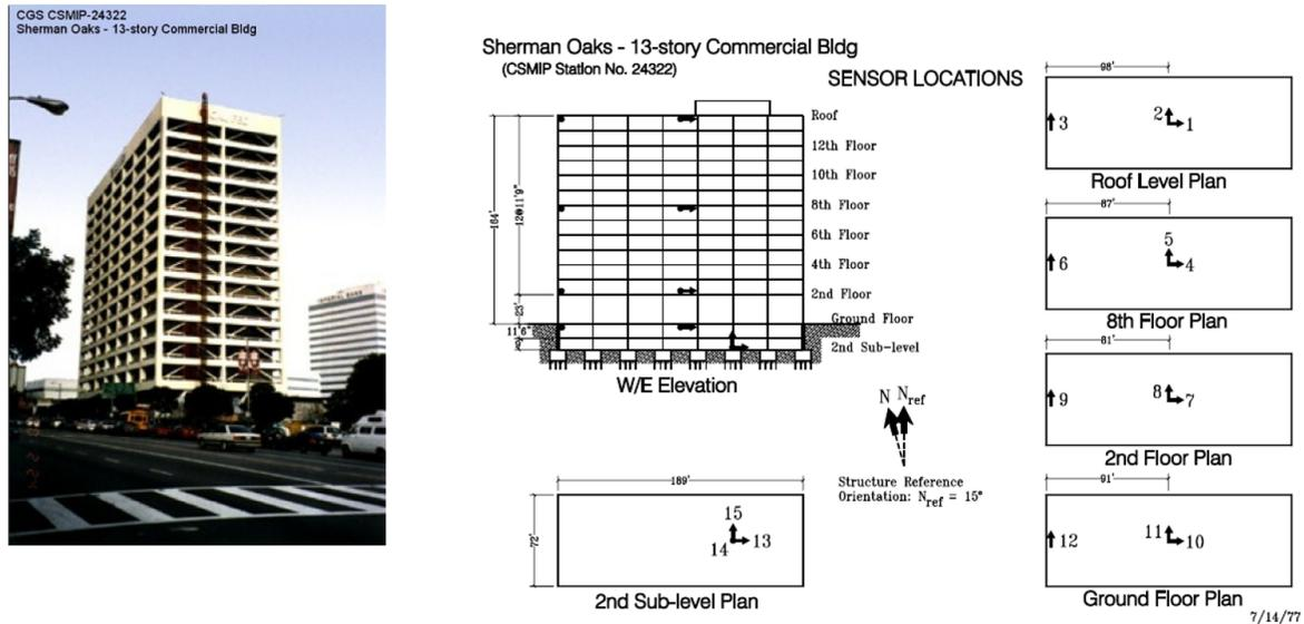
Figure 1: Sherman Oaks – 13-Story Commercial Building, instrumentation layout.
