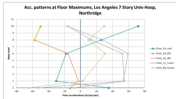
Figure 8: Acceleration values at instrumented floors at the maximum floor acceleration at the individual floor, Los Angeles – 7-Story University Hospital (Base Isolated).
