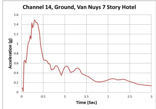
Figure 6: Response spectrum at structure soil interface, Van Nuys – 7-Story Hotel.
