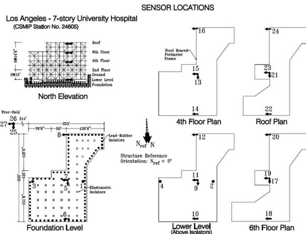
Figure 7: Los Angeles – 7-Story University Hospital, instrumentation layout. Base Isolated building.
