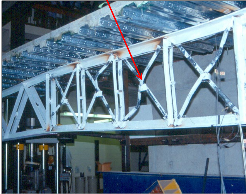
Yielding and buckling of diagonal members
