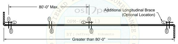
VIII. Each run of pipe requires a minimum of one longitudinal brace. However, a transverse brace placed on the run section at the opposite side of an elbow or tee within 24" may act as a longitudinal brace, and is labeled a "DUAL USE" brace. See layout example below.
