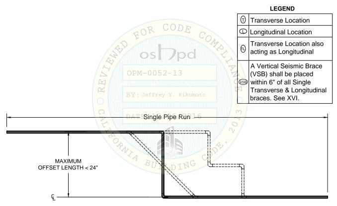
NOTE: When a run of pipe that requires bracing transitions down to a size that does not, the point of transition is considered the end of the run and will require a transverse brace. For an offset less than 24", this is still considered a single run of pipe.
