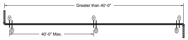
VII. Each pipe run must have at least one longitudinal brace. If the maximum allowable longitudinal spacing is exceeded then add longitudinal braces to meet the spacing requirement.
