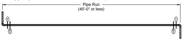
VI. If the distance between the two transverse braces exceeds the maximum allowable spacing, add transverse braces as needed.
