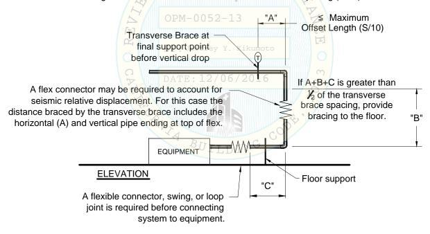
XI. When systems cross a building seismic separation or seismic joint they must be capable of accommodating the joint displacements as specified by the engineer of record.
