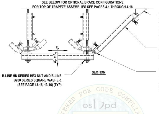
TOLCO FIG. 980, 909, 910, OR 986 **SWAY BRACE ATTACHMENT.** TIGHTEN UNTIL BREAK-OFF BOLT HEAD COMES OFF. (SEE PAGE 12-1, 12-11, 12-12, 12-5)
