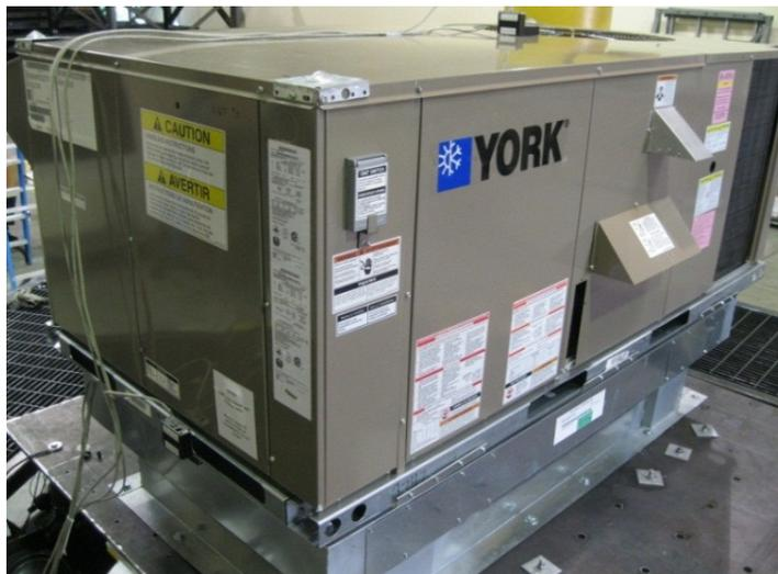
UUT3b was tested on an isolated roof curb by MicroMetl. The curb had six 10-gage anchoring pockets, three on each long side of the curb. The unit was attached to each of the pockets using four #12 1-1/2-inch TEK screws. The curb was attached to the 3/4-inch thick steel shake table interface plate with sixteen 1/2-inch diameter Grade 5 bolts, six each long side and four each short side, with each side sharing a bolt on the corners.
