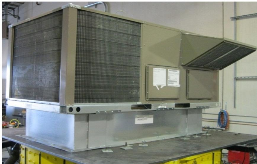
UUT4a was tested on a rigid roof curb by MicroMetl. The curb had six 10-gage anchoring pockets, three on each long side of the curb. The unit was attached to each of the pockets using four #12 1-1/2-inch TEK screws. The curb was attached to the 3/4-inch thick steel shake table interface plate with sixteen 1/2-inch diameter Grade 5 bolts, six on each long side of the curb and four on each short side, with each side sharing a bolt on the corners.
