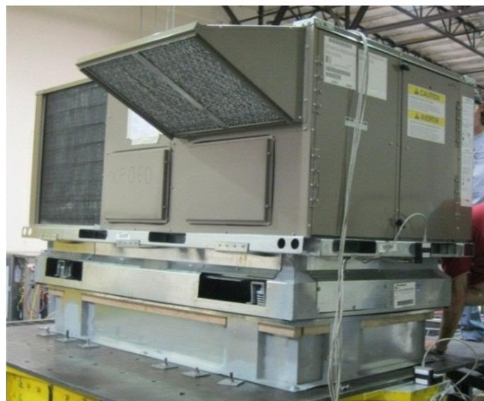
UUT2b was tested on an isolated roof curb by ProVent. The curb had six 12-gage anchoring pockets, three on each long side of the curb. The unit was attached to each of the pockets using four #12 1-1/2-inch TEK screws. The curb was attached to the 3/4-inch thick steel shake table interface plate with six 1/2-inch diameter Grade 5 bolts, one centered at each corner and one centered on each of the long sides of the curb.
