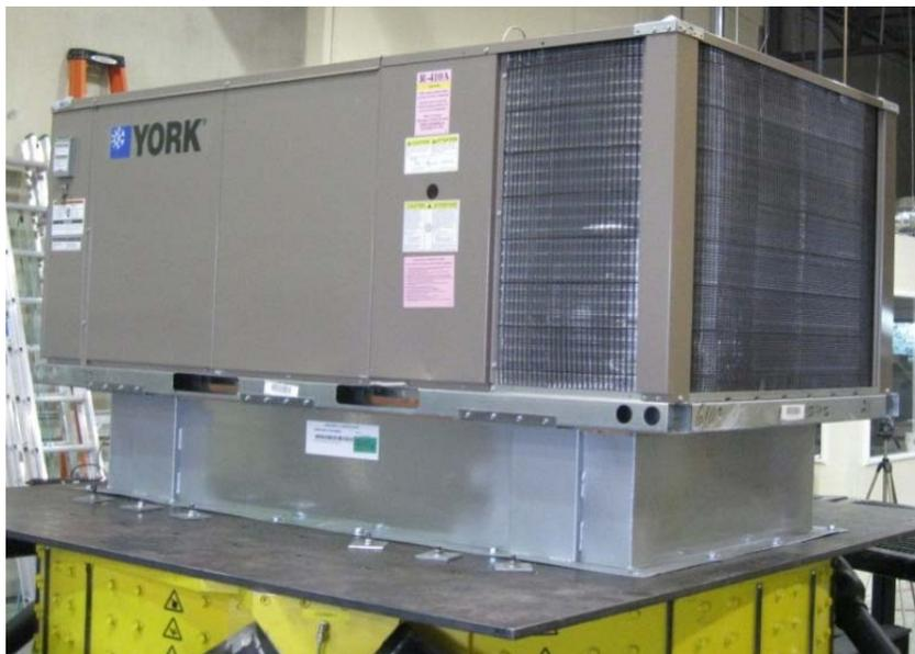
UUT1a was tested on a rigid roof curb by MicroMetl. The curb had six 10-gage anchoring pockets, three on each long side of the curb. The unit was attached to each of the pockets using four #12 1-1/2-inch TEK screws. The curb was attached to the 3/4-inch thick steel shake table interface plate with sixteen 1/2-inch diameter Grade 5 bolts, six on each long side of the curb and four on each short side, with each side sharing a bolt on the corners.
