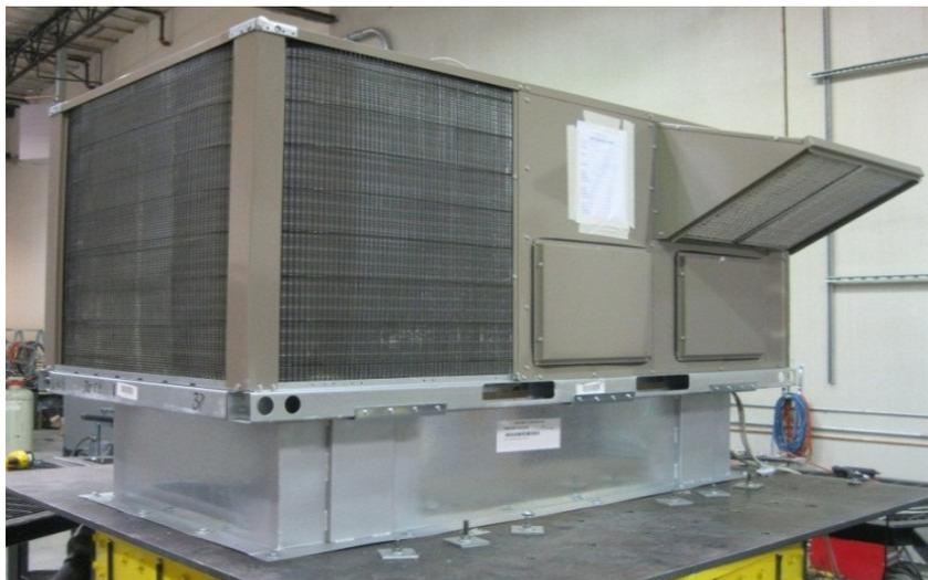
UUT2a was tested on a rigid roof curb by MicroMetl. The curb had six 10-gage anchoring pockets, three on each long side of the curb. The unit was attached to each of the pockets using four #12 1-1/2-inch TEK screws. The curb was attached to the 3/4-inch thick steel shake table interface plate with sixteen 1/2-inch diameter Grade 5 bolts, six on each long side of the curb and four on each short side, with each side sharing a bolt on the corners.
