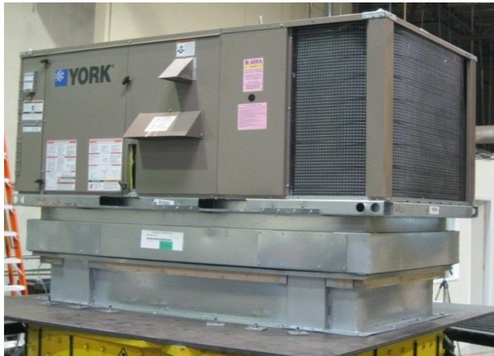
UUT5b was tested on an isolated roof curb by MicroMetl. The curb had six 10-gage anchoring pockets, three on each long side of the curb. The unit was attached to each of the pockets using four #12 1-1/2-inch TEK screws. The curb was attached to the 3/4-inch thick steel shake table interface plate with sixteen 1/2-inch diameter Grade 5 bolts, six each long side and four each short side, with each side sharing a bolt on the corners.
