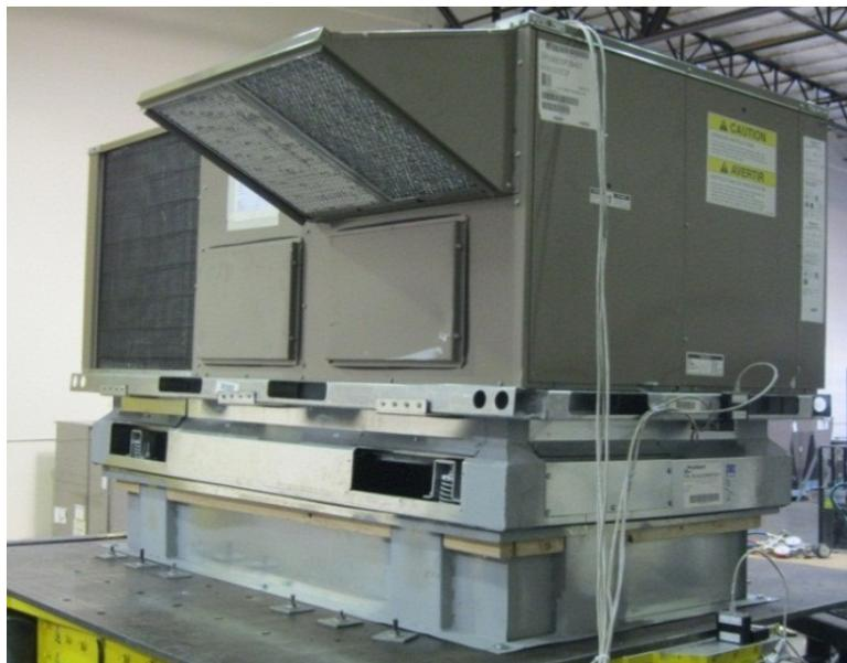
UUT1b was tested on an isolated roof curb by ProVent. The curb had six 12-gage anchoring pockets, three on each long side of the curb. The unit was attached to each of the pockets using four #12 1-1/2-inch TEK screws. The curb was attached to the 3/4-inch thick steel shake table interface plate with six 1/2-inch diameter Grade 5 bolts, one centered at each corner and one centered on each of the long sides of the curb.
