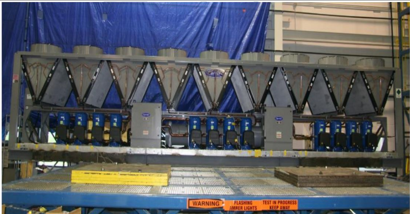
Figure 3: Unit on the shake table
