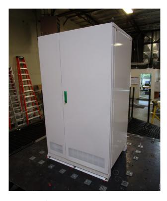
The unit was rigidly mounted at its base with (6) 1/2" diameter Grade 8 bolts, torqued to 80 ft-lb.
