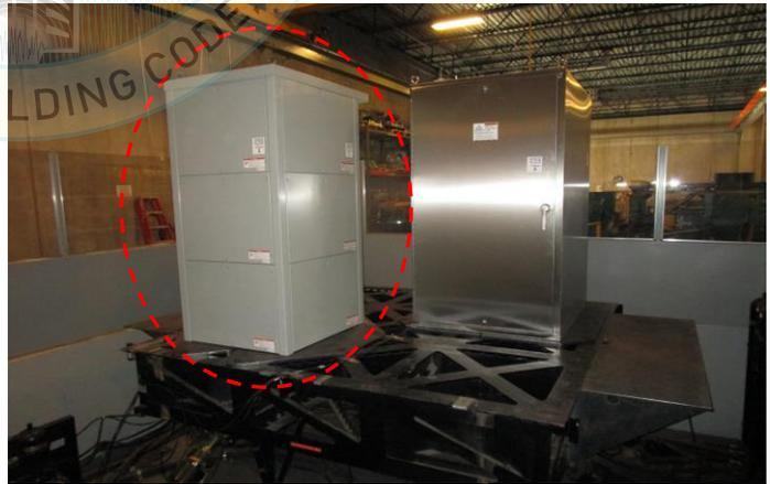
Unit was rigid mounted to test fixture using twelve (12) 3/8" Grade 8 bolts with 1/2" plate washers and 3/8" flat washers. Unit maintained structural integrity and remained functional per manufacturer requirement after shake table test. Contents were included in testing per operating conditions.
