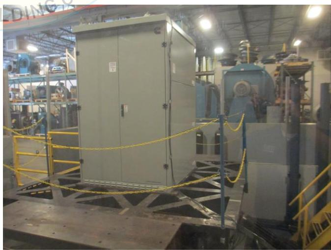
Unit was rigid mounted to test fixture using twelve (12) 3/8" Grade 8 bolts with 1/2" plate washers and 3/8" flat washers. Unit maintained structural integrity and remained functional per manufacturer requirement after shake table test. Contents were included in testing per operating conditions.
