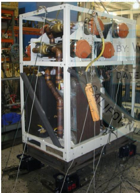
Figure 2B.1: Unit on the shake table
