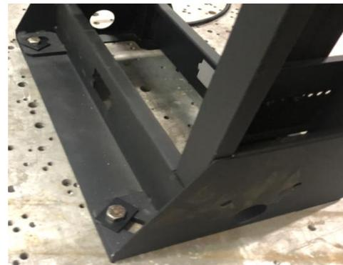
The configuration rack was mounted rigid using four (4) 5/8" - 11 Grade 8 Hex Bolts and Lock Washer and Square Washer. Unit maintained structural integrity and remained functional per manufacturer requirement. Contents were included in testing per operating conditions.
