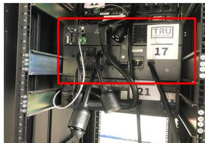
UUT 3c was mounted within a 4-Post Seismic Rack (PN: GL840EZ-3042). UUT 3c was mounted to the rack within the cabinet with a Vertiv rack slide kit (PN: RMKIT18-32). Eight (8) M5 screws and clips, provided by Great Lakes, were used to secure the UUT to the rack.
