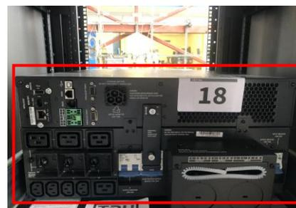
UUT 3d was mounted within a 4-Post Seismic Rack (PN: GL840EZ-3042). UUT 3d was mounted to the rack within the cabinet with a Vertiv rack slide kit (PN: RMKIT18-32). Eight (8) M5 screws and clips, provided by Great Lakes, were used to secure the UUT to the rack.
