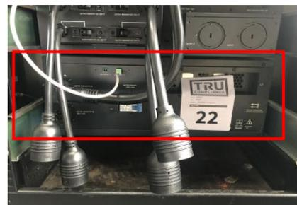
UUT 3g was mounted within a 4-Post Seismic Rack (PN: GL840EZ-3042). UUT 3g was mounted to the rack within the cabinet with a Vertiv rack slide kit (PN: RMKIT18-32). Eight (8) M5 screws and clips, provided by Great Lakes, were used to secure the UUT to the rack.
