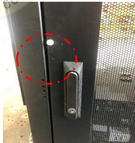
UUT 4 was mounted rigid using four (4) 5/8" - 11 Grade 8 Hex Bolts and Lock Washer and Square Washer. Doors sesimically modified with a #12 self tapping screw.
