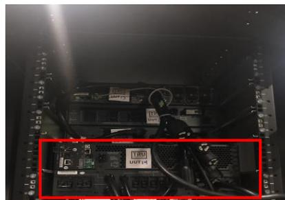
UUT 4b was mounted within a 4-Post Seismic Rack (PN: GL840EZ-3042). UUT 4b was mounted to the rack within the cabinet with a Vertiv rack slide kit (PN: RMKIT18-32). Eight (8) M5 screws and clips, provided by Great Lakes, were used to secure the UUT to the rack.
