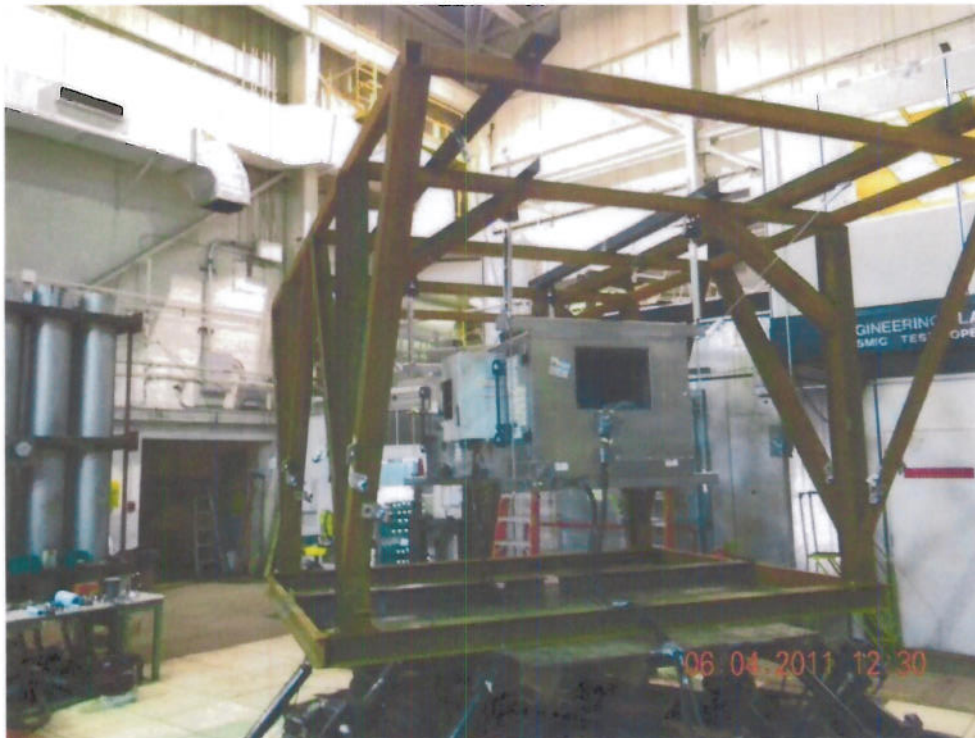
Figure 1. Trane BF-1 PCC Size 6 AHU mounted on Tri-axial Table
