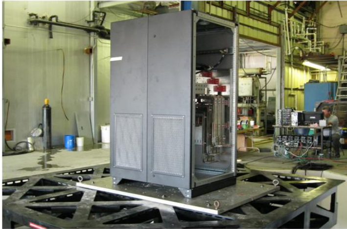
UUT #1 Cabinet is Mounted Directly to the Table Using (4) 5/8" Diameter ASTM A490 Bolts
