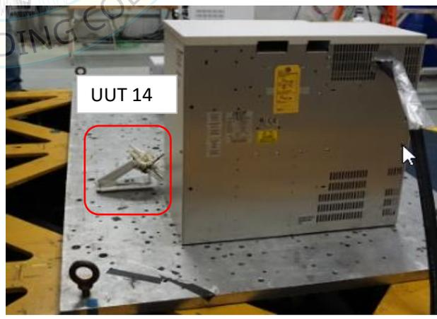
The console bracket base of UUT 14 was mounted to the shake table with two 1" x 4" strips of 3M Dual Lock Reclosable Fastener (P/N TB3550). The mini console of UUT 14 was attached to the bracket with one 1" x 3" strip of 3M Dual Lock Reclosable Fastener. Unit maintained structural integrity and remained functional per manufacturer requirement after shake table test. Contents were included in testing per operating conditions.
