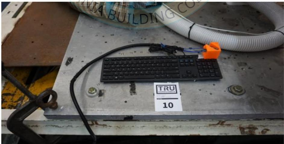
UUT 10 was mounted to the shake table with two 1" x 3.75" strips of 3M Dual Lock Reclosable Fastener (P/N TB3550). Unit maintained structural integrity and remained functional per manufacturer requirement after shake table test. Contents were included in testing per operating conditions.
