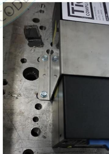
UUT 7 was base mounted – rigid to the table with a custom stainless-steel sheet metal mounting bracket and four #14 x 1-1/2" self-tapping screws. Mounting holes were located at the four corners of the bracket. Unit maintained structural integrity and remained functional per manufacturer requirement after shake table test. Contents were included in testing per operating conditions.
